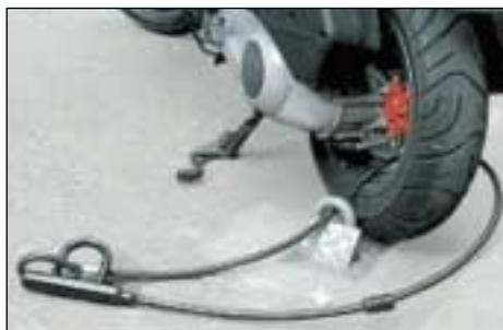
Fig 58: Secure ground level anchor point.
